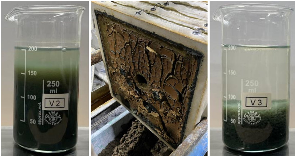
without ZetaPol 1113-Clear = poor sludge quality
